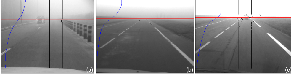
Figure 3. Black segments: measurement bandwidth. Curve on the left: vertical variation of intensity within the bandwidth. Horizontal line: image line representative of the meteorological visibility distance.
