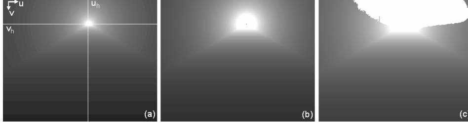
Figure 4. Construction of the depth modeling for the test image of Fig. 3a. (a) a cylindrical scene where a small value of \kappa is assumed. (b) a cylindrical scene where a bigger value of \kappa is assumed, resulting in a larger road surface than in Fig. 4a. (c) The sky region has been added.
