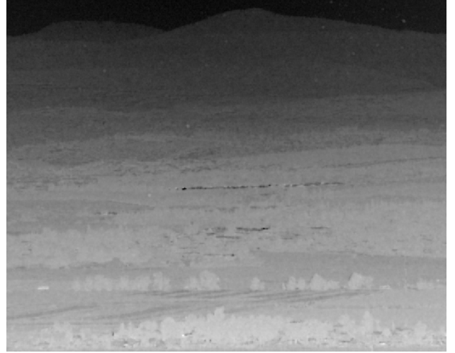
Figure 8. The estimated path radiance. Dark pixels indicate higher path radiance and a larger distance to the objects shown in Fig. 5.
