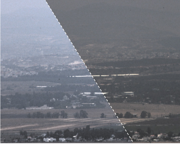
Figure 5. Real polarization filtered images taken in a hazy day. [Left] I^{\max} . [Right] I^{\min} .
