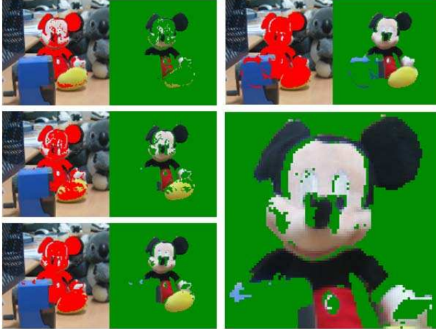
Figure 2. Segmentation results by binarization of RGB color difference. 4 results are selected among lots of results generated by various thresholds. In each pair, the left image describes pixels on the target object by red color and the segmented result is shown in the right. Lower right image shows zoomed part of bottom left which is the best one among them.
