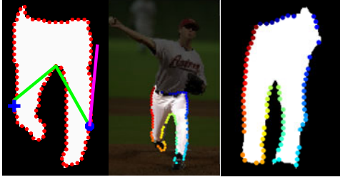
Figure 5. IDSC Computation. Left: We show: shortest interior path (green) from start (blue dot) to end (blue cross); boundary contour points (red); contour tangent at start (magenta). The length of interior path is the inner-distance; the angle between contour tangent and the start of the interior path is the inner-angle. Center: Lower body mask parse; colored points indicate correspondence established by IDSC matching with exemplar on right .
