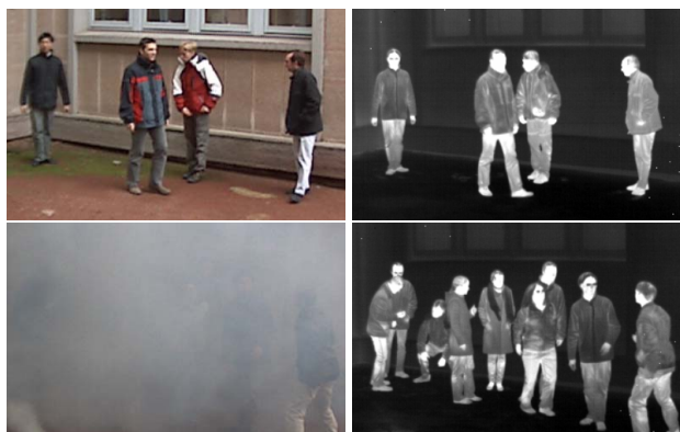
Figure 1. Influence of smoke in both color and thermal images. First row: no smoke, second row: area filled with smoke.
