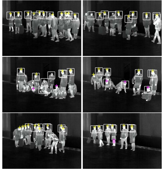
Figure 9. Results of head detection. Crosses indicate head found by local maxima and elliptical shape detector (in yellow above the height threshold, and in magenta below), boxes represent the head detection results obtained with the cascade classifier. The last picture is an example of false detection on legs which presents high gradients.
