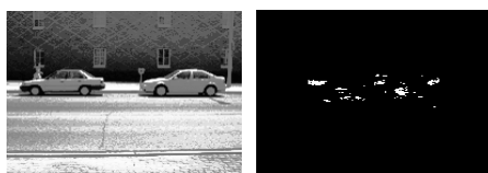
Figure 8 Area template matching result for an input image
