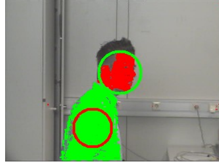
Figure 1. Backprojection maps for face and upper body, overlaid on the original image. For display purposes, the maps were thresholded and pixels exceeding the threshold colored red (face) and green (upper body). The circles represent the estimated size (only for the face) and center of the tracked region
