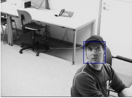
Figure 2. KLT features and their scores (0%-100%), shown as pixels of increasing brightness
