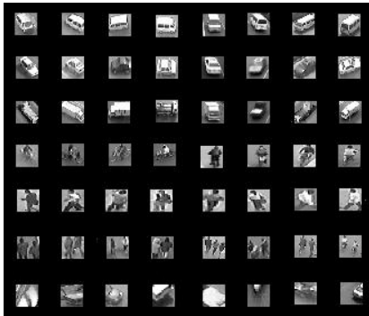
Figure 6. Some examples of training samples. The training set contains van, car, truck, bike, person, group of people and spurious object, which are collected in diverse camera viewing angles.
