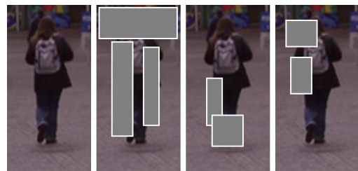
Figure 10. Top three composite Haar features automatically discovered. The top one composite feature, shown in the second left image, indeed looks like a person with two legs. For the second composite feature, one component lands on the foot, and the other lands on a leg. These are all important areas for people detection. Note that only the bounding boxes of the Haar features are displayed for clarity.
