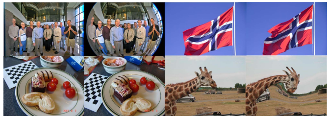
Figure 1. Examples of image pairs with various deformations in our experiments: The left image pair of the first row images are with fisheye lens deformation, the right image pair of the first row images with nonrigid deformation, the left image pair of the second row images with affine deformation, and the right image pair of the second row images with synthetic deformation.
