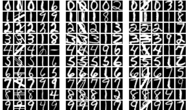
Figure 6. Denoising USPS scratched digit images. Each 5-tuple is composed of, from left to right, (1 st ) the noise-free test image, (2 nd ) randomly scratched image, (3 rd ) denoised by NN on COIR, (4 th ) NN on KSIR, and (5 th ) NN on the scratched image x itself.
