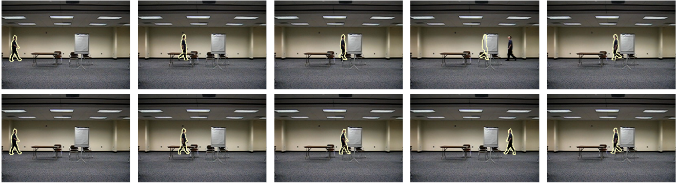
Figure 4. Local versus global optimality. Image segmentation with a dynamical shape prior, implemented by gradient descent (top row) and by Lipschitz optimization (bottom row). While gradient descent can handle partial occlusion by the table, it fails to handle total occlusion (4th image). The proposed Lipschitz optimization, on the other hand, guarantees the globally optimal solution and therefore reliably tracks the person upon reappearing from behind the white board.
