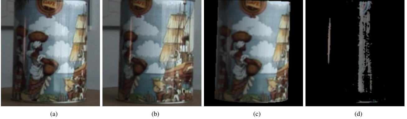
Figure 4. Estimation of texture and reflections. (a,b) First and last frame of a video sequence. (c,d) The diffuse and specular images computed as described in Section 3.2. Image (d) was gamma-corrected for clarity.
