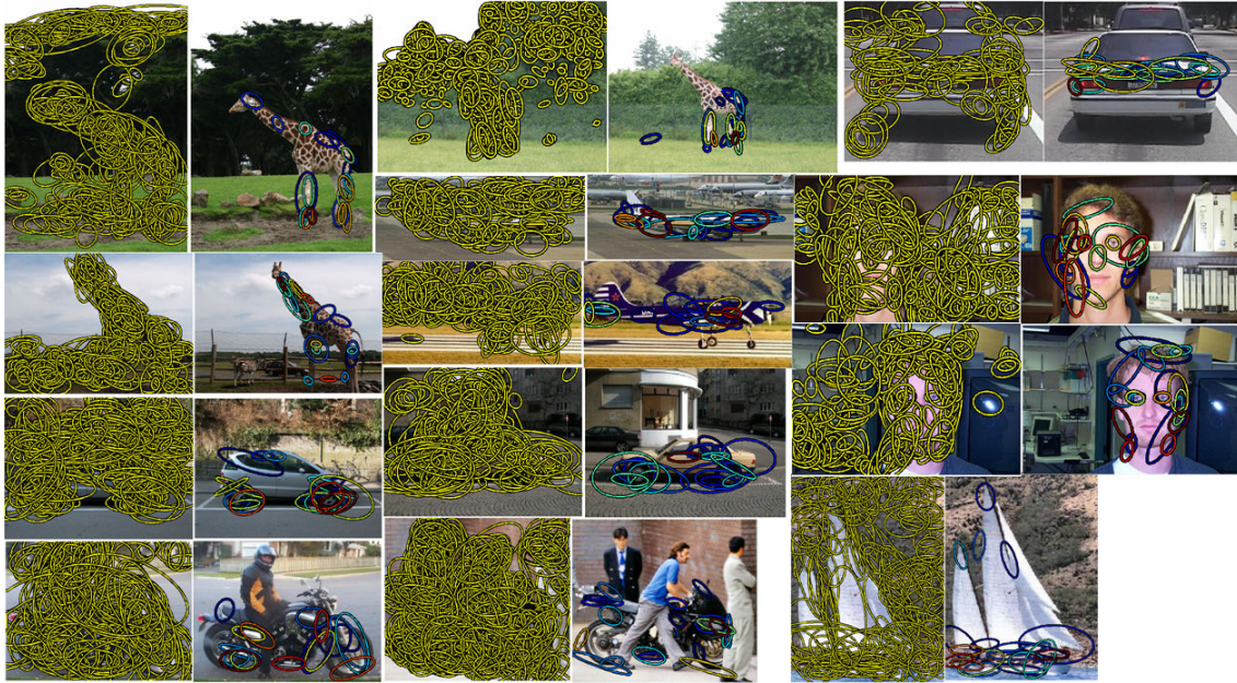
Figure 5. Some examples of localization for the Caltech-101 and TUD/ETHZ dataset. In each image pair, the left image represents original extracted features with yellow, and the right image shows top 20% high-ranked features with color variance according to the importance weights. The jet colormap is used from red(high) to blue(low). (These figures are best viewed in color.)
