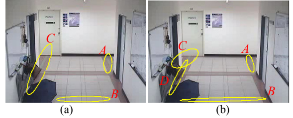
Figure 3. An example of entry/exit zone estimation for Cam 3 in Figure 6. (a) the entry/exit zones, A , B , and C , after batch learning phase. (b) the entry/exit zones, A , B , C , and D , after adaptive learning phase. Note that zones C and D are very close. The zone C in (a) is split and adapted to zones C and D in (b) incrementally.
