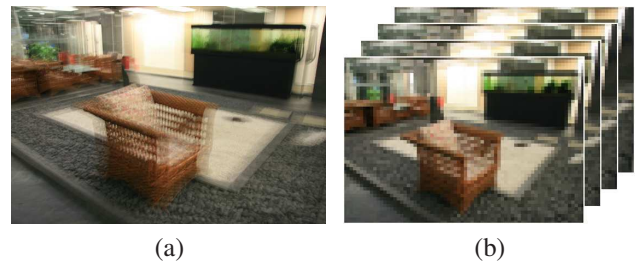
Figure 1. Tradeoff between resolution and frame rates. (a) Image from a high resolution, low frame rate camera. (b) Image from a low resolution, high frame rate camera.
