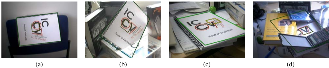
Figure 9. Accuracy of the retrieved transformation. For each of these images, we draw the borders of the book estimated from a single patch. This is made possible by the fact we estimate a full perspective transform instead of only an affine one.
