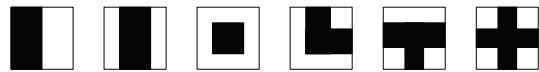
Figure 3. Some image primitives for sketchable areas. Image primitives are composed of +1's and -1's and allowed to rotate in 8 directions.
