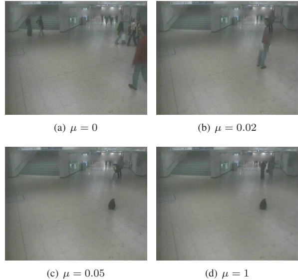
Figure 4. Background estimated with the cost function of [1], using “minimum contrast” image objective weighted by different \mu 's.
