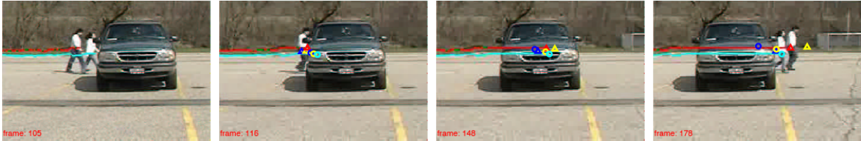
Figure 7. Track matching with overlapping tracks and a moving camera: comparison between Kalman filter (blue circle and triangle), CF and Particle filter (yellow circle and triangle), and our approach (cyan circle and red triangle).
