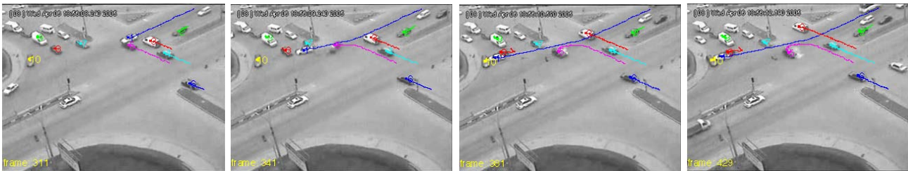
Figure 11. Crash detection. Tracks of 10 cars in frame 311, 341, 381, and 429.
