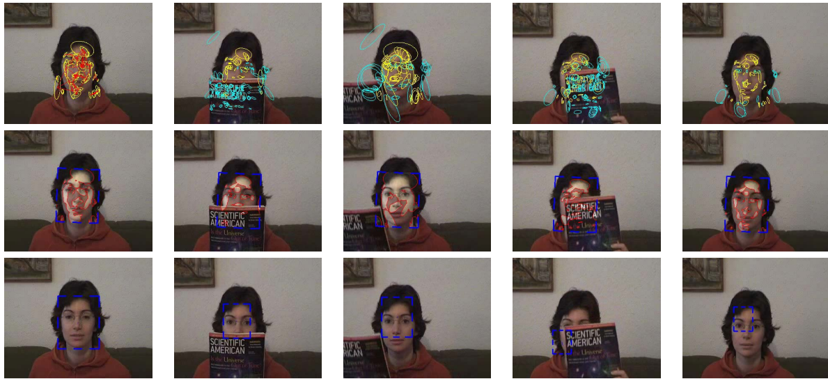
Figure 7. Tracking [Face] for frame #1, 285, 345, 585 and 599, (1st row) initialization and interest region detection, (2nd row) the proposed tracker (3rd) the Mean-shift tracker.
