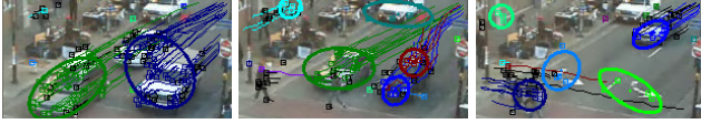
Figure 6. Under- and over-segmentation errors and false detections when the Normalized Cut was directly applied frame-by-frame without background subtraction.
