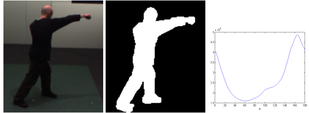
Figure 2. This example image (left) is converted into a silhouette (middle) to which the \mathcal{R} transform (right) can be applied.
