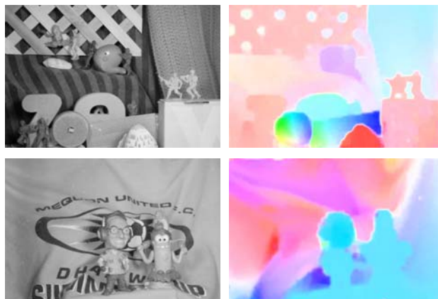
Figure 1: The 10th frame of the Army sequence (upper row) and Mequon sequence (lower row) and our estimated (color-encoded) optical flow fields.
