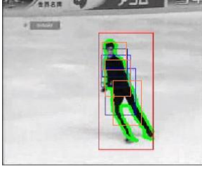
Figure 4. Blue: The block configuration from the previous frame. Green: The contour is estimated using a fast graph-cut algorithm. Red: The blocks are repositioned using a greedy strategy to provide a maximal coverage of the target.
