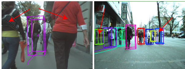
Figure 7. Typical false negatives (pedestrians at large scales) and false positives (reflections, trees) of our system.
