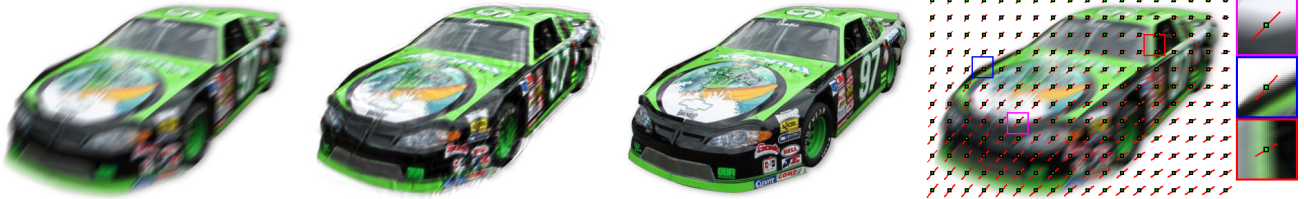
Figure 6. Affine motion from blur with synthesized data. From left to right: affine blurred image, deblur result, ground truth, visualized affine motion field estimation result with close-up views (please notice that the estimated local blur vector match the blur extend precisely).
