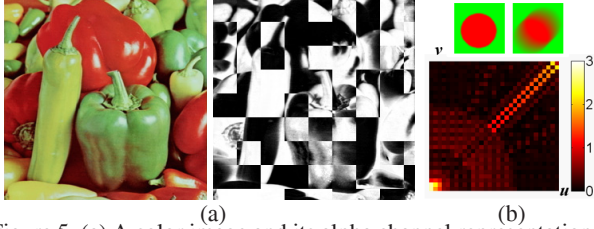
Figure 5. (a) A color image and its alpha channel representation \alpha , (b) top: original unblurred image ( 70 \times 70 ) and one blurred image with \mathbf{b} = (20, 20)^T , bottom: error ( \|\mathbf{b}^* - \mathbf{b}\| ) map of parameter estimation for all \mathbf{b} \in \{(u, v)^T \mid u, v \in \{0, 1, \dots, 30\}\} .
