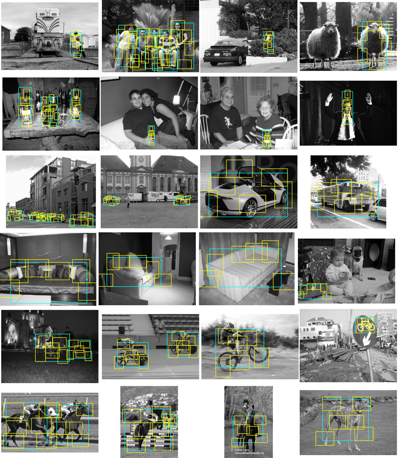
Figure 5. Some results from the PASCAL 2007 dataset. Each row shows detections using a model for a specific class (Person, Bottle, Car, Sofa, Bicycle, Horse). The first three columns show correct detections while the last column shows false positives. Our system is able to detect objects over a wide range of scales (such as the cars) and poses (such as the horses). The system can also detect partially occluded objects such as a person behind a bush. Note how the false detections are often quite reasonable, for example detecting a bus with the car model, a bicycle sign with the bicycle model, or a dog with the horse model. In general the part filters represent meaningful object parts that are well localized in each detection such as the head in the person model.
