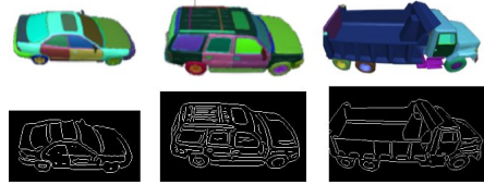
Figure 2. 3D model examples and their representation. Each vertex of a 3D model is represented by both its position and semantic ownership information. We render each part in a unique pseudo color (first row), and the edges between parts are extracted (second row) for shape matching.
