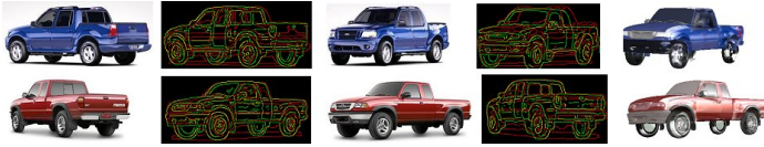
Figure 12. Model selection, pose estimation, and rendering results for two pickup trucks. Col. 1 & 3: Original views; Col. 2 & 4: Model edges projected on image edges, a Mazda B-Series is chosen in both cases; Col 5: Rendered images from Col. 1 to 3.
