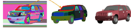
Figure 6. Obtain global semantic part level appearance from image segmentation. For each part segment(such as the red box for the front window), compute the main mode of the color from all the intersecting segments from real image segmentation (left) and assign the appearance. Right column is a global rendering example.
