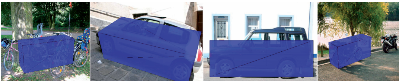
Figure 9. Remaining issues illustrated on a few examples from the PASCAL 06 dataset (from left to right): incorrect feature matches, failed 3D pose estimation, unknown object geometry, not enough features for a successful pose estimation due to the size of the objects. This figure is best viewed in color.
