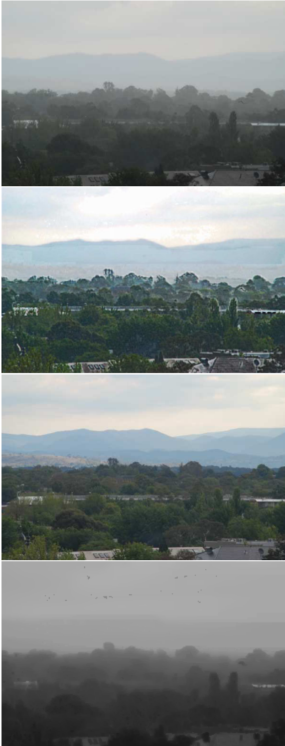
Figure 11. Top: input image. Second from top: the direct attenuation. Third from the top: the ground truth. Bottom: the airlight. Note that, we increase the intensity of the direct attenuation, since the input image is considerably darker than the ground truth.
