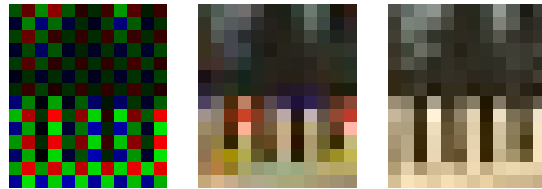
Figure 3. Failure cases of local gradient estimation. From left to right: CFA image, AAI interpolated, ground truth.
