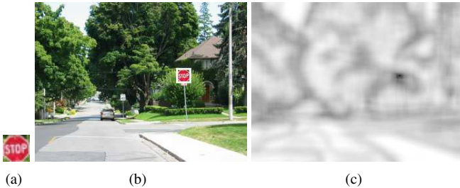
Fig. 7. Traffic sign search example. a) 19 \times 19 target template, b) 320 \times 240 input search image with a bounding box overlaid on the matched target region and c) corresponding L_2 similarity (log scale) image based on a 16^3 -bin (RGB) tensor histogram (darker intensities indicative of greater similarity). The distributive histogram detects the target in 868 msec using 1.25 MB of memory, while the integral histogram takes 5295 msec using 1200 MB of memory.
