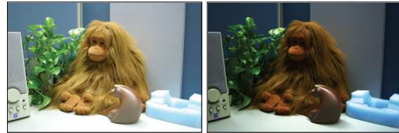
Figure 7. The result of intensity linearization using the estimated camera response functions for Camera D.
