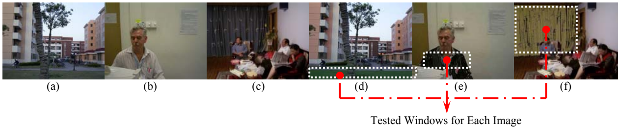
Figure 8. (a-c) 3 real images taken by a DEC U350 camera. (d) It is tampered from (a) in the following places: The kind of bald lawn becomes grass green; the lower part of the rope binding the tree in the middle portion of the photo is adhered to lichen; the street lamp is “lighted”; and the old pink wall of the two apartment buildings at both left and right parts of the photo is “repainted”. (e) The man is clothed with a black sweater, outside his stripped T-shirt originally in (b). (f) The curtain at the rear of the room in (c) is colored with brown yellow. The tested windows are suspicious and cropped for detection.
