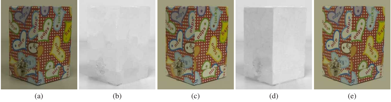
Figure 1. Box. (a) Original image. (b)-(c) Shading and reflectance image without the use of texture cues. (d)-(e) Shading and reflectance image with our non-local texture algorithm.
