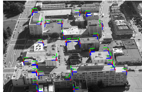
Figure 9. 134 correct DSM-image matches after GMSAC: blue intersections denote image 2DOCs, green intersections denote projected DSM 2DOCs, and red lines indicate the correspondence between them.
