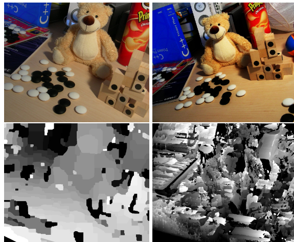
Figure 1. Depth maps for view-based synthesis: Top row: Two 800 \times 600 calibrated images we use as input. Bottom row: On the left, the depth map computed using DAISY and on the right, depth map computed using normalized-cross correlation, which could not handle the large perspective and contrast change between the two input images.
