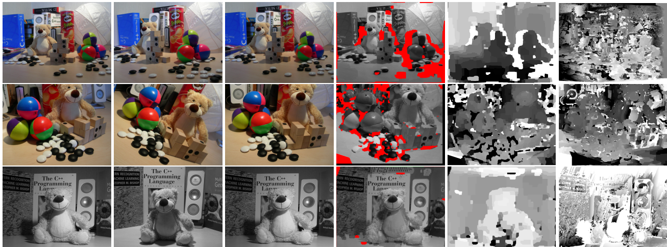
Figure 9. Depth maps and resynthesized images. In each row, the first two images are the inputs to our stereo-matcher. The third one is not used to compute the depth but only to validate the quality of the fourth one, which is synthesized from the first two using the DAISY depth map shown in fifth position. The final image is the depth map computed using normalized cross-correlation. The occluded areas are overlaid in red in the synthetic images. Note that in the last row, the two input images were lit differently which slightly degrades the performance but nevertheless allows credible resynthesis.
