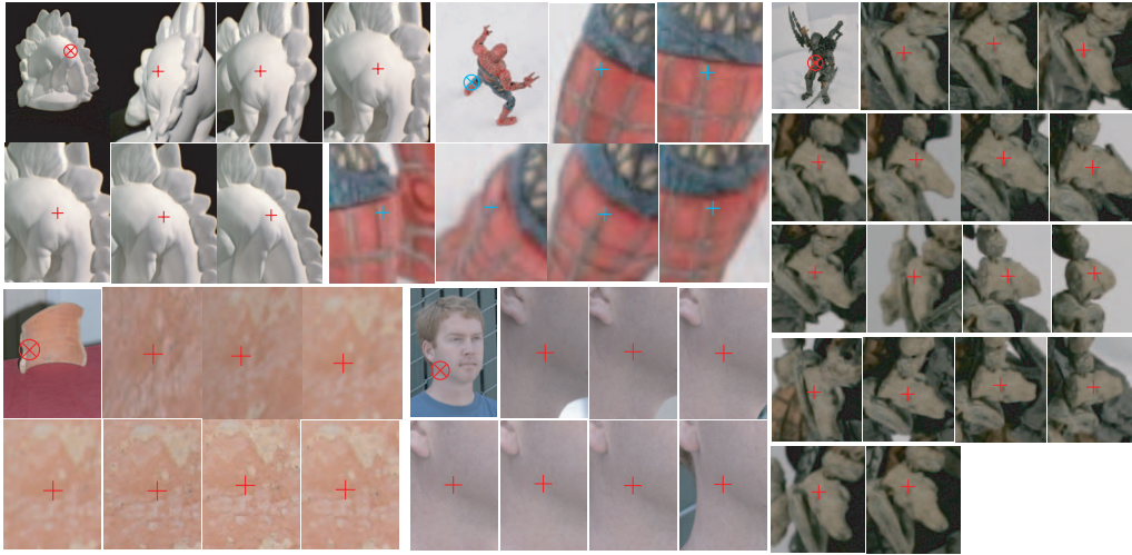
Figure 6. A set of matching 2D features is shown for each dataset. The proposed method is able to match features in many images even without salient textures due to the use of surface geometry and visibility information estimated by the multi-view stereo algorithm.
