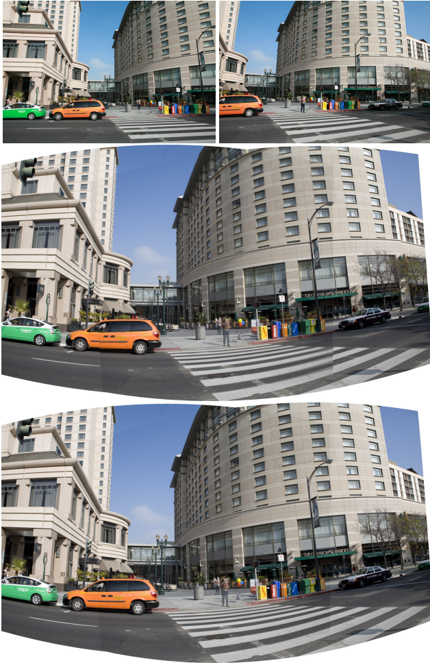
Figure 3. Comparison on real images with and without lens distortion estimation: The top row was two input images. The middle row was the result obtained without lens distortion estimation. We can see visible mis-alignments in the crosswalk region. The bottom row was the result obtained with lens distortion estimation. The improvement in alignment quality is clear.
