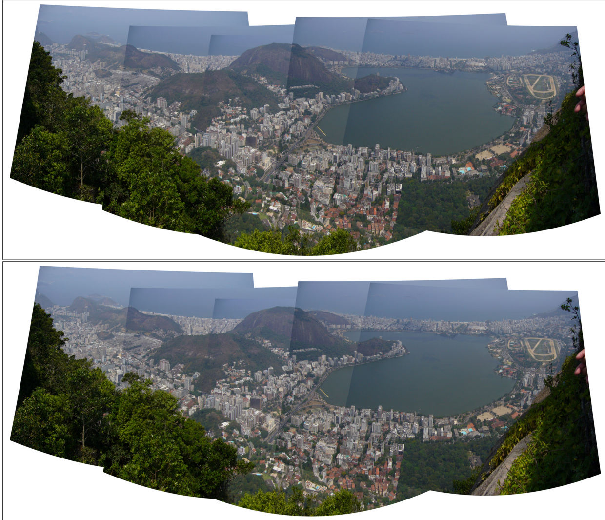
Figure 4. Importance of multi-image bundle adjustment: The first composite is created with pairwise bundle adjustment but without multi-image bundle adjustment while the second is created with both types of bundle adjustments. One can observe that the alignment is better in the second composite.
