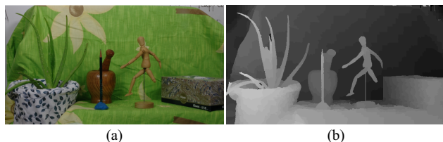
Figure 5. Result from Puppet image pair. (a) Original left image and (b) depth map ( \alpha_{th} = 0.5 ).
