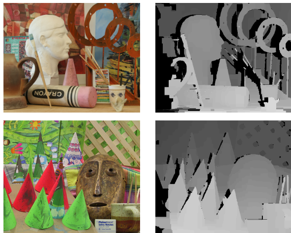
Figure 1. Sample disparity maps for stereo scenes Art and Cones produced by long-range CRF models ( K = 3 ) learnt with l_{occl} loss function. For “Art” (top), the model is trained on the rest 5 scenes in the same data set; for “Cones” (bottom), the model is trained on all 6 scenes in the Middlebury-2005 data set (which contains “Art” but not “Cones”). Occluded regions inferred by the model are masked in full black.
