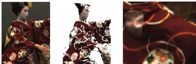
Figure 8. Super-resolution reconstruction of single-view video sequence. (Left) shows an original frame. (Middle) shows the projection of the relevant pixels from 10 consecutive frames onto a blank HR grid. (Right) shows a detail of the super-resolved reconstructed image.
