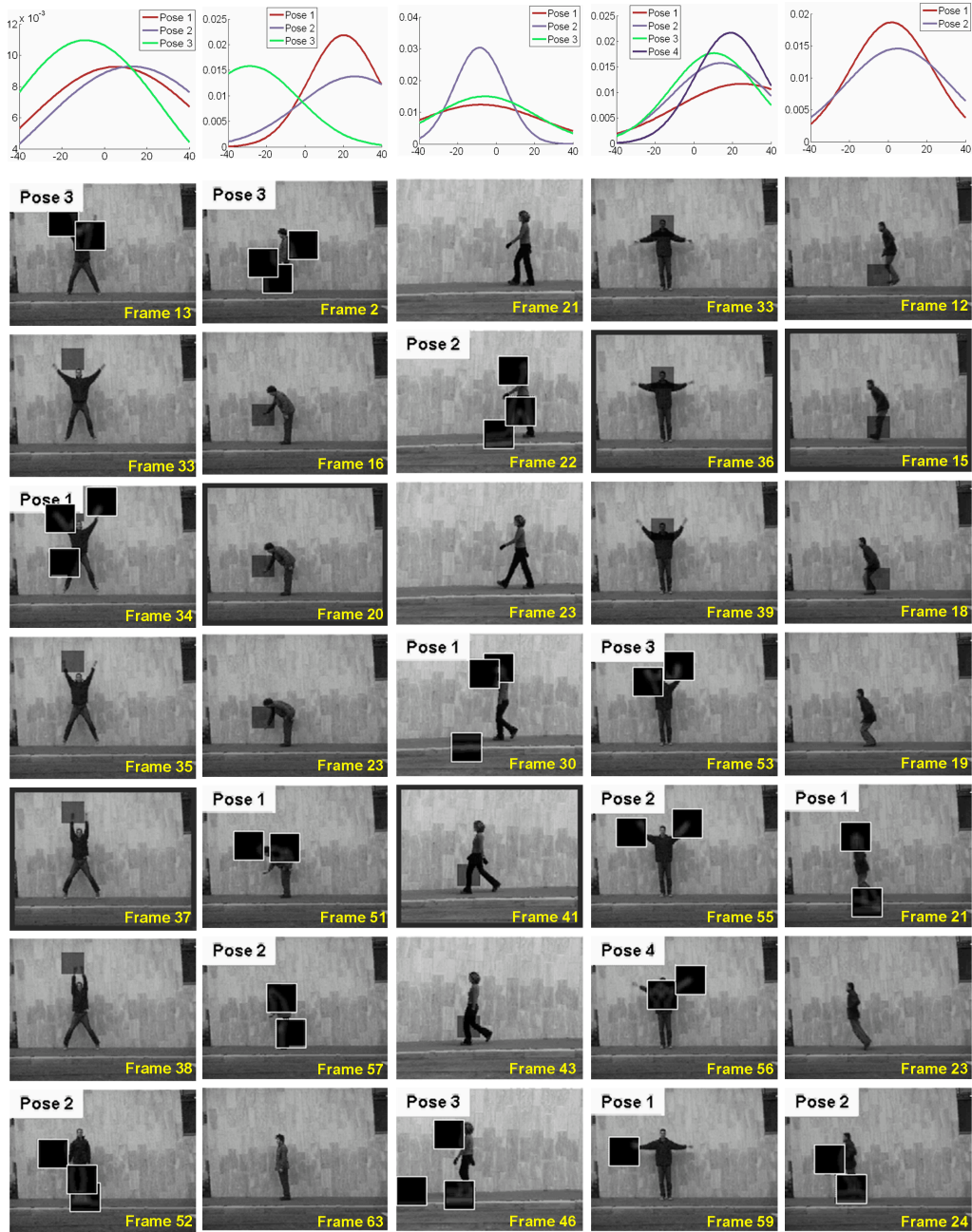
Figure 7. Learned motion models superimposed on the test sequences at the detected locations. White borders indicate static-pose parts. Grayed rectangles represent 2D central slice of the landmark spatio-temporal subregion in corresponding frames. Dark border highlights the temporal coordinate of the spatio-temporal feature corresponding to the landmark node of dynamics.
