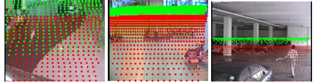
Figure 4. Examples of scene-adaptive grids for large , small , and zero camera tilt angles.
