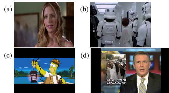
Figure 1: Examples of conventional handling of different aspect ratios for video material and display device. (a) squeezed, (b) cropped, (c) letterboxed, (d) pillarboxed.
