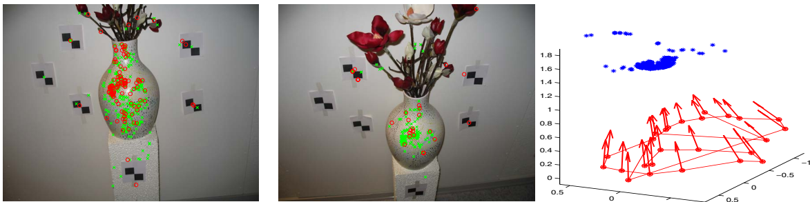
Figure 6. The triangulation problem. Two images (out of 25) with points used for calculating the reconstruction to the right. Green points (inliers) are used for the triangulation while red points are detected as outliers because of miss matchings.
