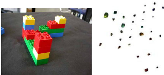
Figure 3. One of the seven images of the Lego sequence (left) and the polyhedral triangulation result (right). The small polyhedra bound the corners of the object.
