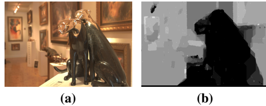
Figure 6. A scene with complex lighting conditions is shown in (a) and the resultant depth map is shown in (b).
