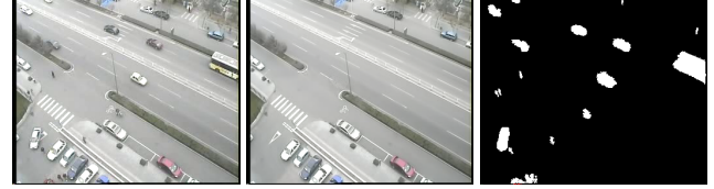
(a) One frame of videos (b) Background recovered (c) Detected moving objects
